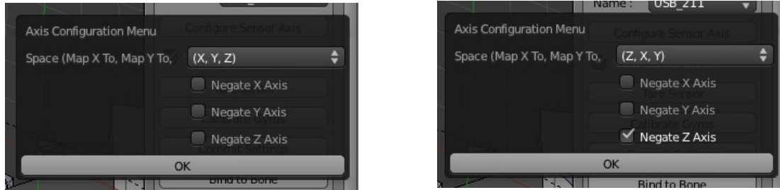
A “before and after” look at the Axis Configuration Menu. It has been changed to reflect the needed axis directions for the example.
